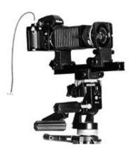
combination (for example, a 50mm tube divided by a 200mm lens focal length equals an 0.25X or 1/4-life-size "magnification").
